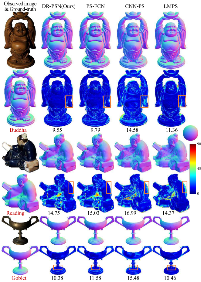
Fig. 6. Qualitative results for real-world scenes from the DiLiGenT benchmark dataset with 10 sparse input images. The black numbers under the error maps represent MAE( ^{\circ} ). The contrast of the observation images are adjusted for easy viewing in the same parameter (50% enhancement). The orange boxes in the error maps are the regions with cast shadows. Our method produces more robust estimations in these regions.
