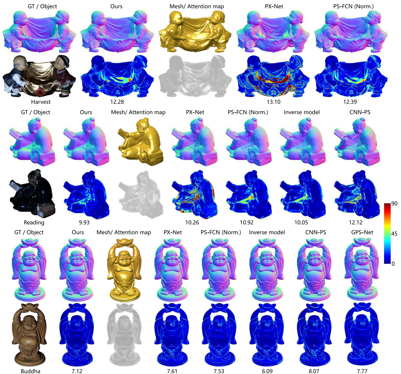
Fig. 10 Quantitative results on objects “Harvest”, “Reading”, and “Buddha” on the DiLiGenT benchmark data set (Shi et al., 2019), with 96 input images. The third column shows the 3D reconstruction results of our estimated surface normal maps using (Simchony et al., 1990) and
