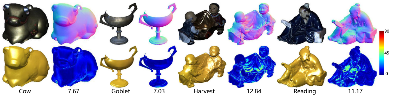
Fig. 13 Quantitative results on the objects “Cow”, “Goblet”, “Harvest”, and “Reading” in the DiLiGenT test data set (Shi et al., 2019) with 96 input images
